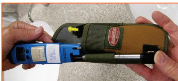
**Figure 2. EC probe inserted into resistor on holster to check calibration (Doran & Kucera, 2012).**
