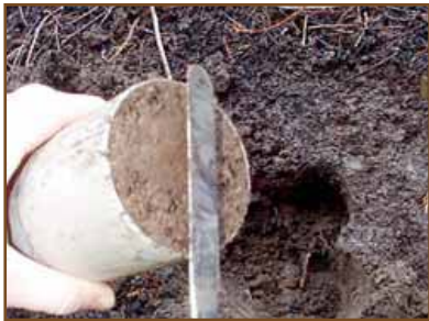
Figure 8. Remove excess soil from bottom of ring.
