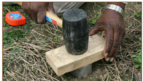
Figure 6. Drive ring to 3-inch depth.
