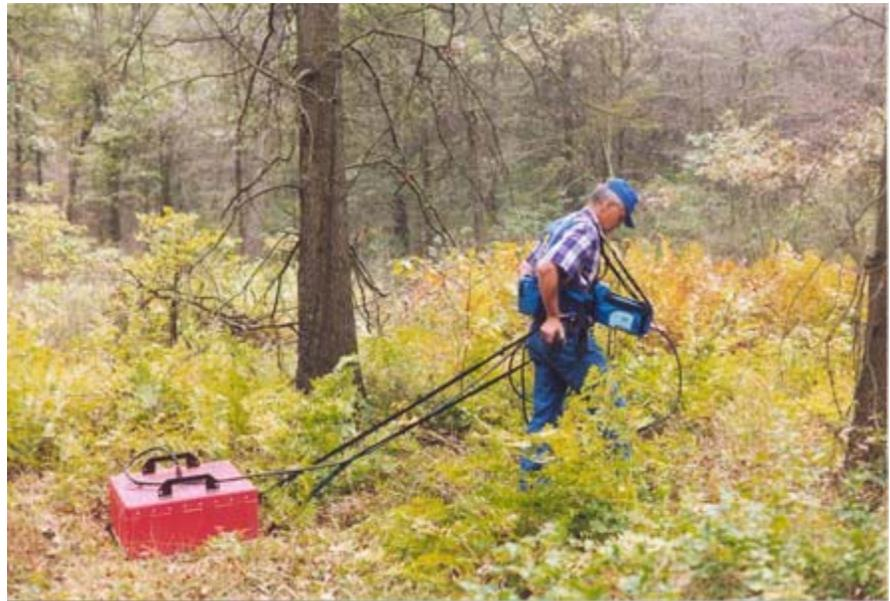
Jim Doolittle taking onsite measurements by means of ground-penetrating radar.
