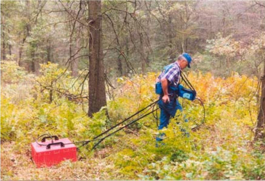
Onsite measurement by means of ground-penetrating radar.
