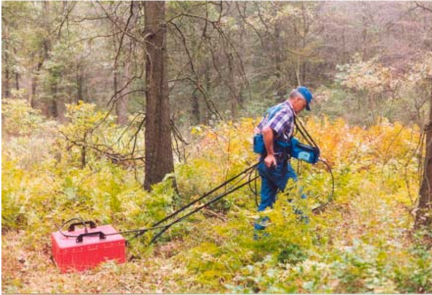
Onsite measurement by means of ground-penetrating radar.
