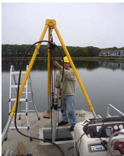
Jim Turenne, Rhode Island Assistant State Soil Scientist, demonstrates the use of a vibracore to collect a subaqueous soil core.
