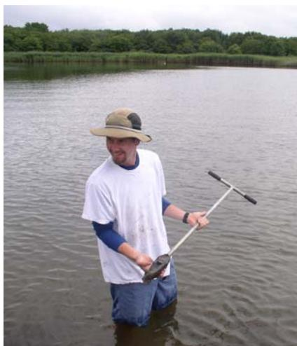
The tools used in mapping soils in shallow water commonly are the same as those used in mapping terrestrial soils, such as augers.
