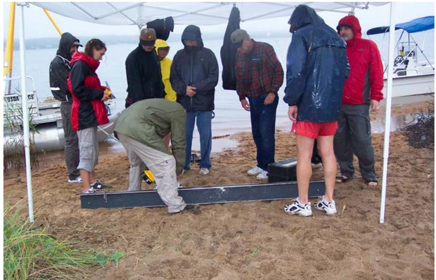
NRCS staff from the National Soil Survey Center and from Connecticut and Rhode Island cutting a vibracore open at Ninigret Pond.
