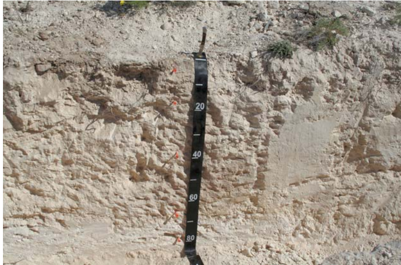
Profile of a classic gypseous soil. This soil has more than 40 percent gypsum throughout.
