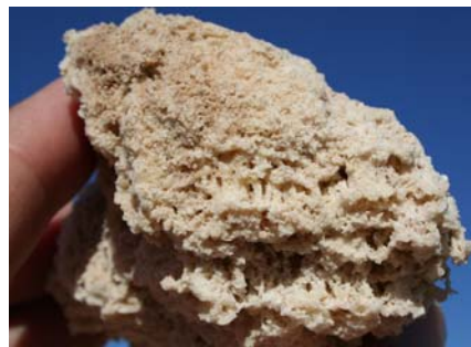
Honeycomb gypsum, a porous cemented layer, appears to exhibit precipitation and dissolution soil-forming processes.
