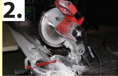
**2.** Cut strips into 3-inch pieces using miter saw (tin snips work for small projects). To reduce splintering, use a fine-toothed plywood blade (200 teeth), vinyl siding blade, or tile saw blade (**Caution: Always follow manufacture’s guidelines for safety when operating power tools**). Multiple undersill strips can be stacked and cut at once to expedite production. Cut slowly.
