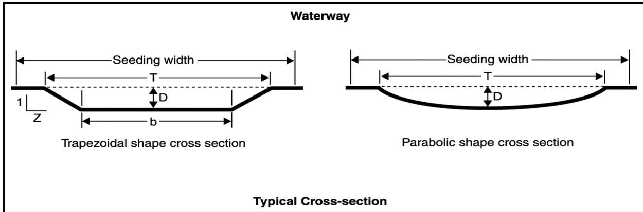
A grassed waterway can have a cross-section configuration that is trapezoidal or parabolic. Side slopes are constructed to be no steeper than a ratio of two horizontal to one vertical. The intent is to accommodate maintenance and tillage/harvesting equipment that will cross the waterway. Waterways are generally less than 100 feet wide to control the tendency of low flows to meander.
