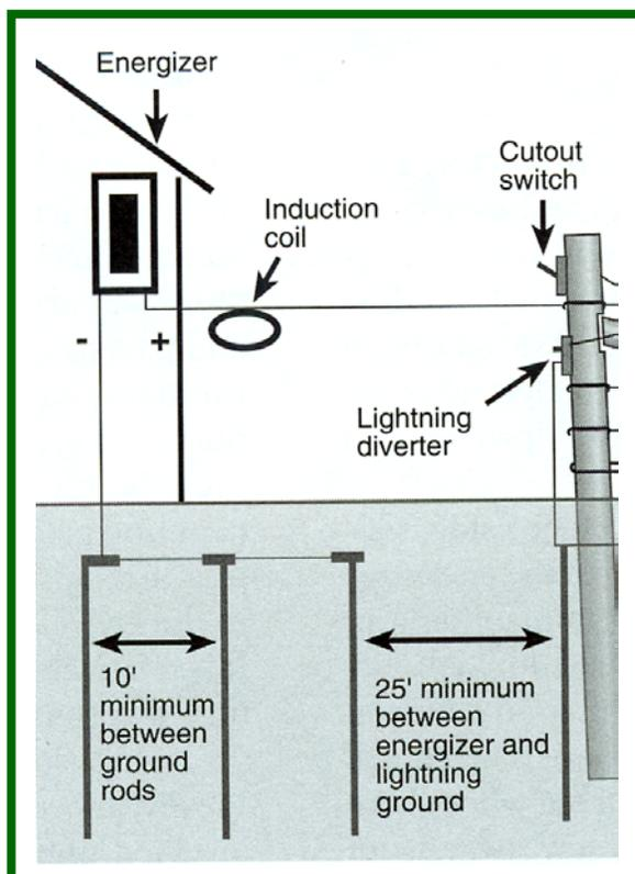
*The effectiveness of an electric fence depends in large part on an adequate grounding system.*
