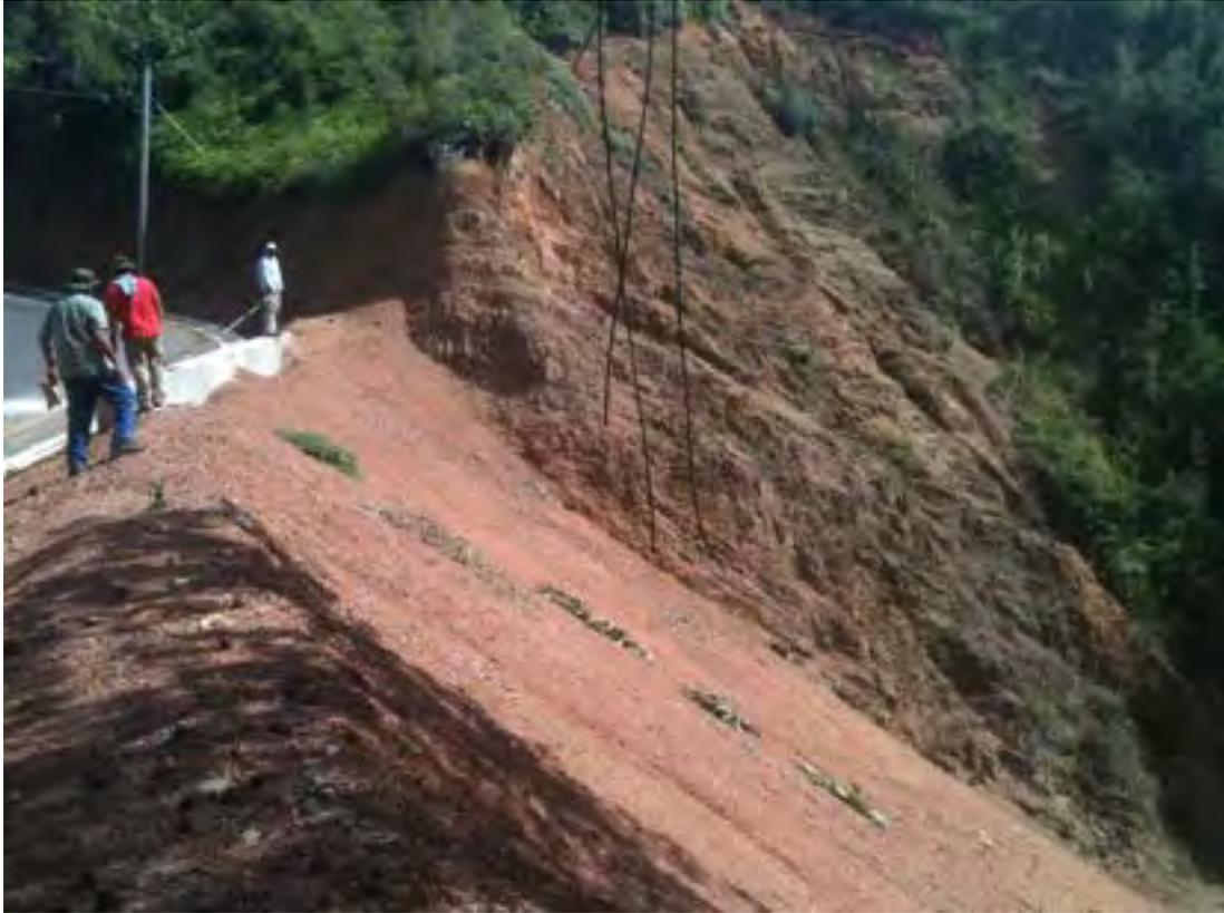
Figure 1. Laying out test plots on a 70-75% slope
