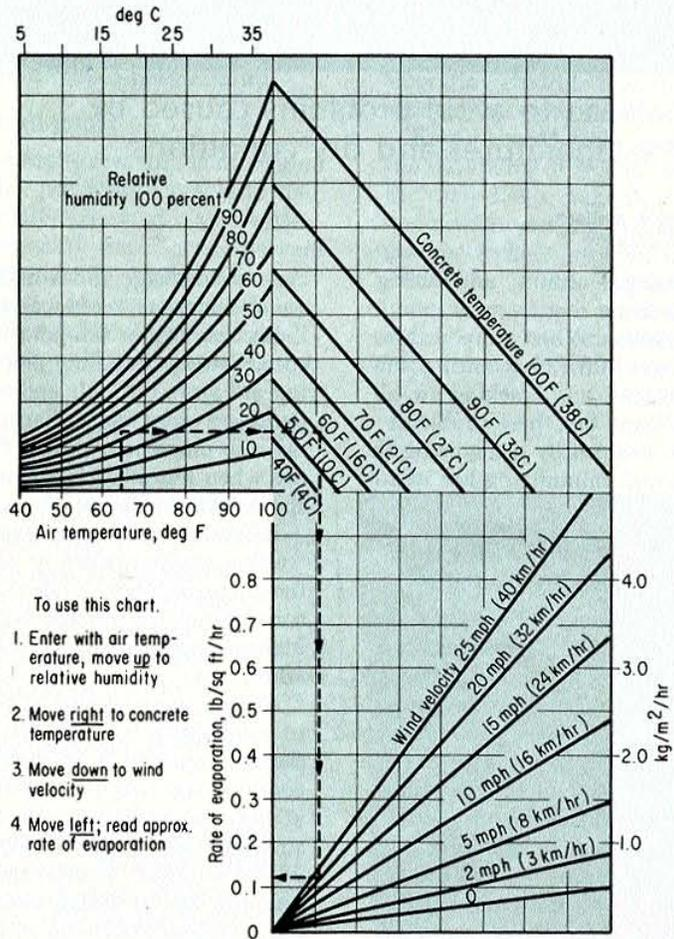
Figure 2. Use this chart to estimate evaporation rate from concrete surfaces. Plastic shrinkage cracking is possible if the rate exceeds 0.1 pound per square foot per hour. When the rate exceeds 0.2 pound per square foot per hour, take steps to slow surface evaporation. Steps may include cooling the concrete, using a fog spray, or using windbreaks. (Chart is found in ACI 305-89, Hot Weather Concreting.)
