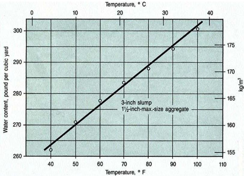
Figure 1. At higher temperatures, more water is needed to produce a given slump. (Data from U.S. Bureau of Reclamation)
