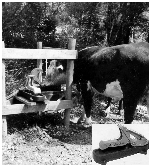
Figure 4. This nose pump uses animal power to pump water from a stream to the watering cup.
