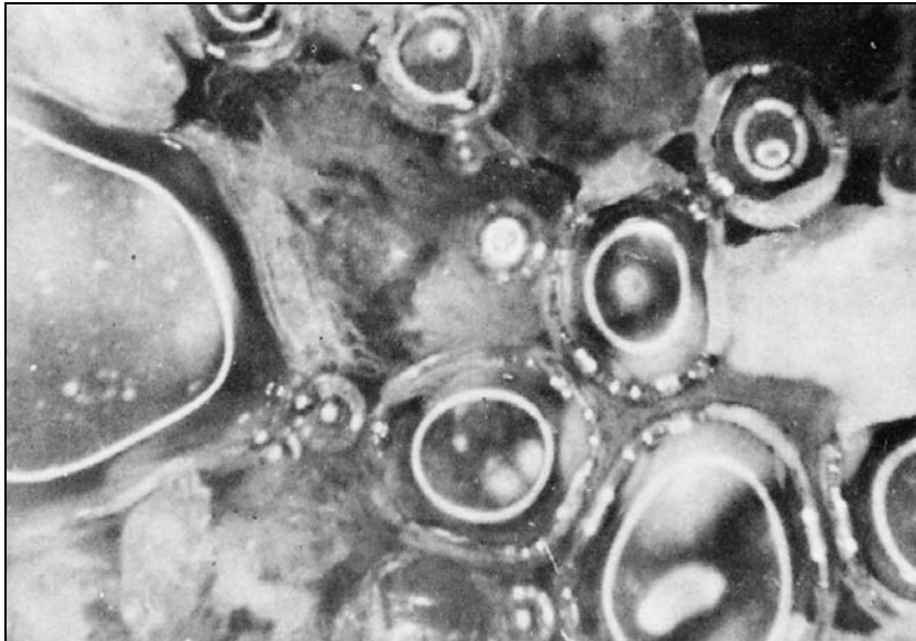
This photomicrograph of air entrained plastic concrete suggests how minute bubbles of air function as very small ball bearings which make the concrete more workable than a non-air entrained mix.
