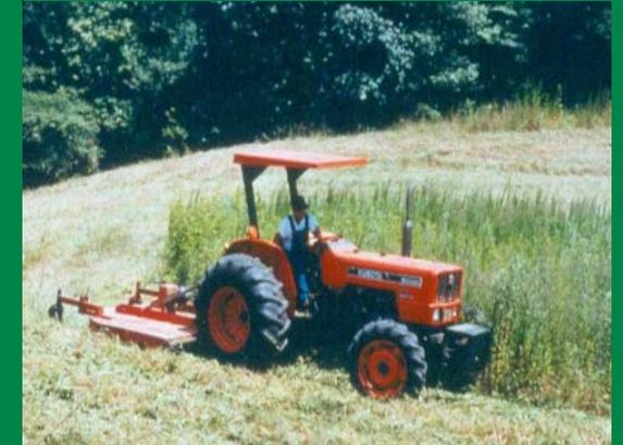
*Fertilizing and mowing vegetation on embankments and spillways is important.*
