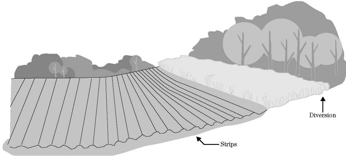
**Figure 4-4** Interceptor drain on bottom land
