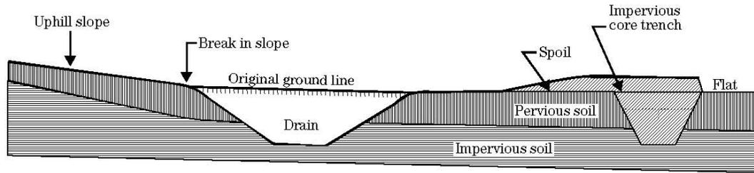
**C.** - Cross section showing open drain as surface water diversion and subsurface water interceptor located at interface of sloping and flat lands.
