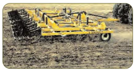
FOR RUSLE2 CALCULATIONS THIS IS TWO OPERATIONS—FIELD CULTI-VATOR WITH COILED TINE HARROW.
