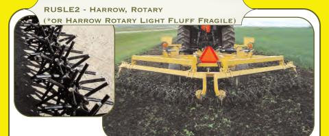
TINES DISTURB ONLY THE TOP INCH OR SO OF SOIL. IN GENERAL, THE GREATER A TOOL IS ANGLED OFF THE TOOL BAR, THE MORE THAT OPERATION WILL DISTURB THE SOIL. THE PHILLIPS<sup>TM</sup> HARROW IS PERMANENTLY SET AT A 45 DEGREE ANGLE. (DEPENDING ON THE TYPE OF RESIDUE PRESENT, USE HARROW ROTARY FOR HEAVY, NONFRAGILE RESIDUE SUCH AS CORN, AND HARROW ROTARY LIGHT FLUFF FRAGILE FOR LIGHT RESIDUE SUCH AS SOYBEANS.)
