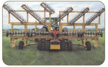
FOR RUSLE2 CALCULATIONS THIS IS TWO OPERATIONS—AERATOR WITH ROTARY HARROW.
