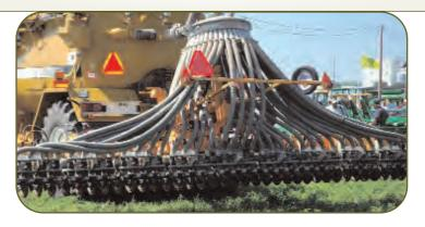
TANK TYPE LIQUID MANURE INJECTOR WITH LOW DISTURBANCE COULTERS. HOWEVER, BECAUSE 15 INCH ROWS ARE USED HERE, THIS METHOD DISTURBS TWICE AS MUCH SOIL SURFACE AS WHEN 30 INCH ROWS ARE USED. AS A RESULT RUSLE2 SOIL LOSS CALCULATIONS WILL BE HIGHER WITH 15 INCH VERSUS 30 INCH UNITS.
