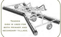
A DISK IS A TILLAGE IMPLEMENT THAT PULVERIZES OR SMOOTHS THE SOIL. ITS CONCAVE CUTTING BLADES ARE MOUNTED ON A COMMON SHAFT TO FORM A GANG. A DISK CONSISTS OF TWO OR MORE GANGS ATTACHED TO A FRAME. THE OPERATING DEPTH IS USUALLY ONE QUARTER OF THE DISK DIAMETER.
