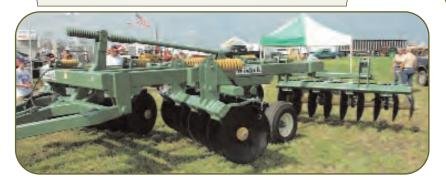
SOMETIMES CALLED A PLOWING DISK, THIS DISK USES ITS WEIGHT AND LARGE DIAMETER BLADES TO SLICE AND TURN SOIL AND RESIDUE. IT DOES EXTENSIVE SOIL DISTURBANCE AND RESIDUE BURIAL.
