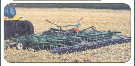
FOR RUSLE2 CALCULATIONS THIS IS THREE OPERATIONS—COULTER CADDY AND A ROLLING CULTIVATOR. NOTE: THIS TURBO-TILL HAS A ROLLING BASKET INSTEAD OF THE COIL TINE HARROW.
