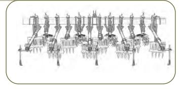
A ROLLING CULTIVATOR USES TWO SPIDER GANGS ON EACH ROW ASSEMBLY. IT OPERATES IN HEAVY RESIDUE WITHOUT CLOGGING.
