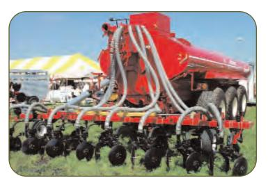
TANK TYPE LIQUID MANURE INJECTOR WITH HIGH DISTURBANCE
