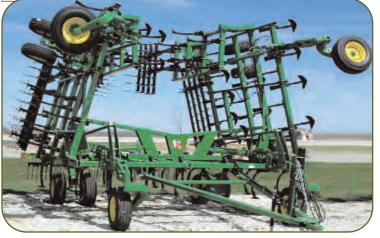
FOR RUSLE 2 CALCULATIONS, THIS IS TWO OPERATIONS—CULTIVATOR, FIELD 6-12 INCH SWEEPS WITH HARROW COILED TIMES.
