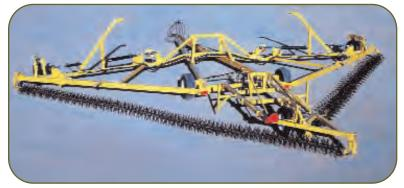
THE PHILLIPS<sup>TM</sup> ROTARY HARROW WORKS IN THE TOP INCH OR SO TO PREPARE SEEDBEDS. IT REDISTRIBUTES RESIDUE AND LEVELS THE GROUND. (\*DEPENDING UPON THE TYPE OF RESIDUE PRESENT, USE HARROW ROTARY FOR HEAVY, NONFRAGILE RESIDUE SUCH AS CORN AND HARROW ROTARY LIGHT FLUFF FRAGILE FOR LIGHT RESIDUE SUCH AS SOYBEANS.)
