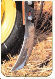
IN THE MIDWEST ANHYDROUS AMMONIA COMPRISES THE MAJORITY OF COMMERCIAL NITROGEN APPLICATION. ANHYDROUS AMMONIA MUST BE INJECTED INTO THE SOIL. THIS IS COMMONLY DONE WITH NARROW KNIVES ATTACHED TO A TOOL BAR PULLED BY A TRACTOR. PRECISE APPLICATION IS IMPORTANT FROM ECONOMIC AND ENVIRONMENTAL PERSPECTIVES.
