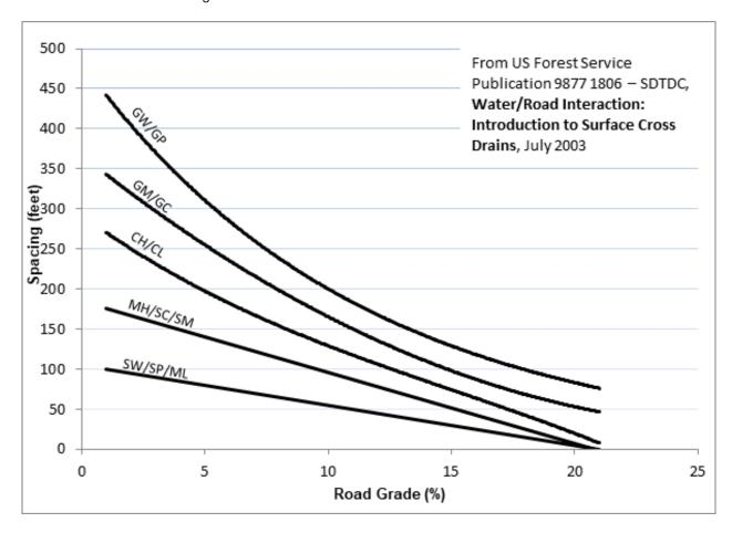
Figure 1. Minimum spacing for surface cross drains for trails or walkways with exposed soil, by soil type (Unified Classification System).
