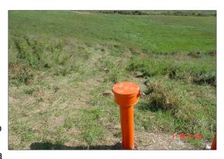
water well and a monitoring well is the monitoring well must be built so that water entering the well is only from the soil or rock layers of interest.
