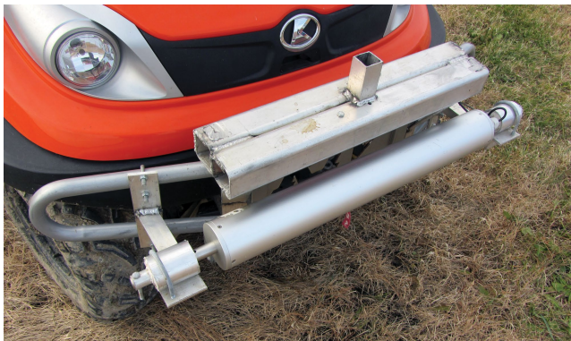
A vehicle-mounted passive gamma-ray sensor.
