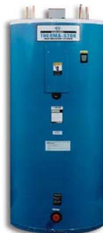
Compressor Heat Recovery units, also called refrigeration heat recovery units, are used to capture waste heat from the milk refrigeration system and utilize it to heat water. The benefits of a compressor heat recovery system can be reduced if used in conjunction with a plate cooler because the amount of waste heat available for use by the heat recovery system is reduced.
