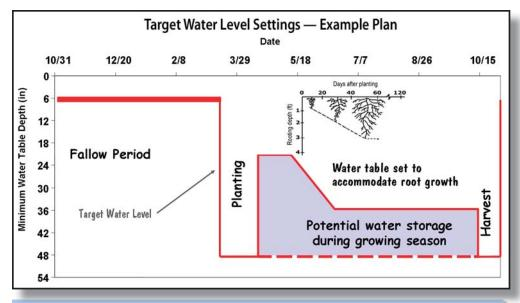
DWM is the process of managing timing and amount of water discharges from agricultural drainage systems. The DWM plan provides the target water table level settings needed at specific dates or seasons.
