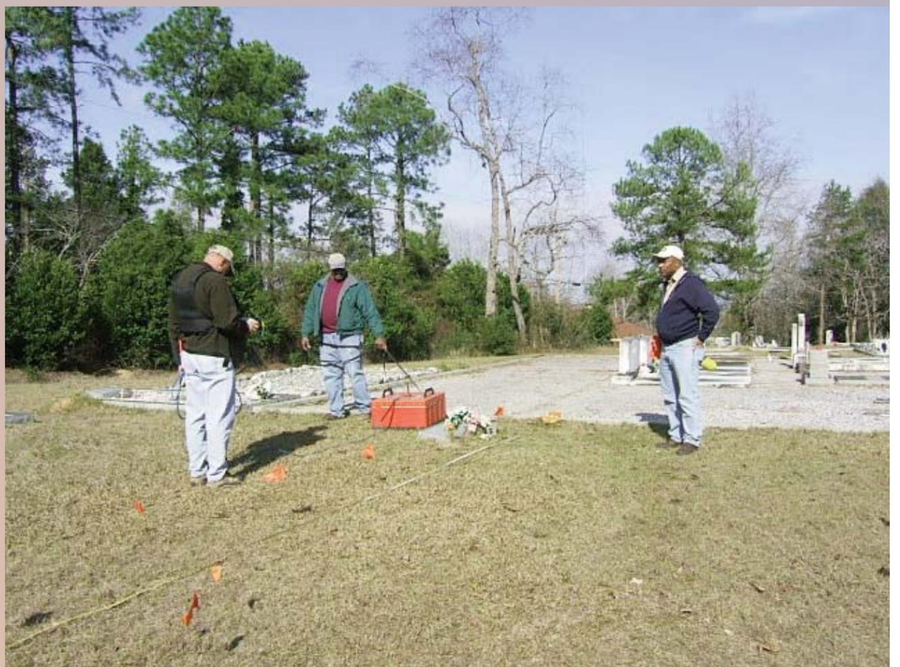
The Ground Penetrating Radar unit is pulled along a line of flags as the operator looks for disturbances in the soil profile which indicates a potential gravesite.
