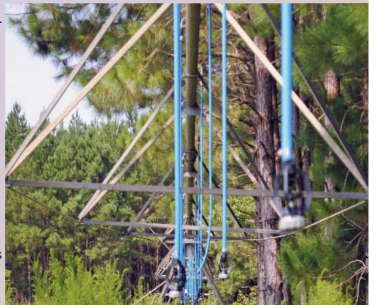
The center pivot irrigation system on Dasher’s farm were retrofitted to low pressure hoses and now operates on an electric pump as well.
