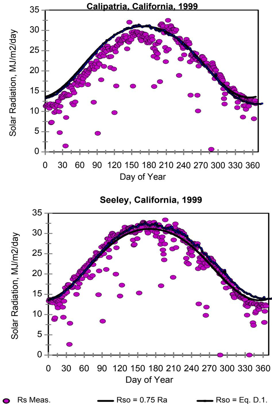
Figure D-1. Daily Measured  $R_s$  and Calculated  $R_{s0}$  using Eq. 19 of the text and using Eq. D.1 – D.5 for Calipatria (top) and Seeley (bottom), California CIMIS stations in the Imperial Valley during 1999.
