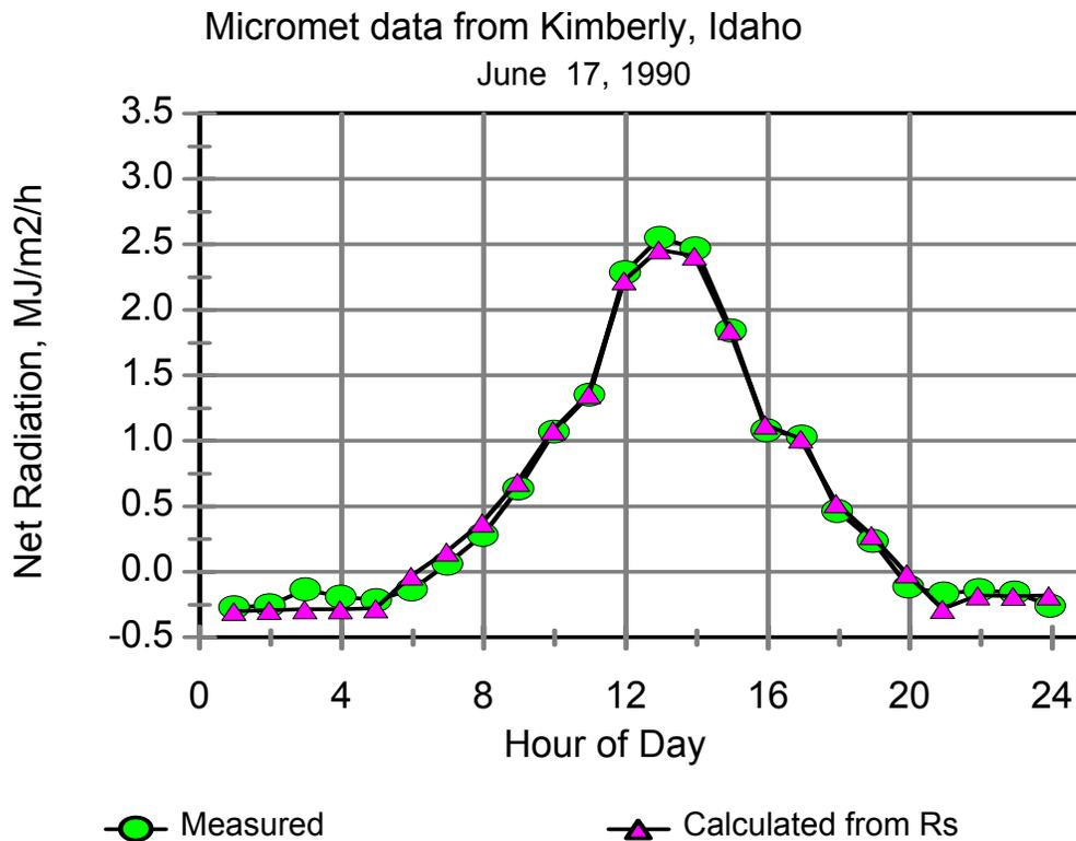
Figure D-4. Measured and calculated hourly net radiation for one day at Kimberly, Idaho over clipped grass ( $R_n$  was calculated using Eq. 42-60). Data courtesy of Dr. J.L. Wright, USDA-ARS, Kimberly.
