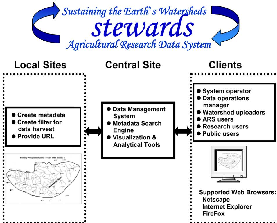
Figure 2. Architecture of the ARS STEWARDS data system.
