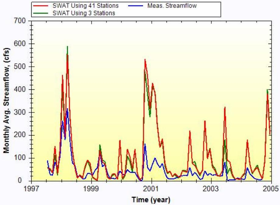
**Figure 6.** Comparison of simulated monthly streamflow for Scenario #1, 41 rain gages, and #3, 3 rain gages, to measured streamflow. (Results for Scenario #2, 21 rain gages, were not distinguishable from those of scenario #1).
