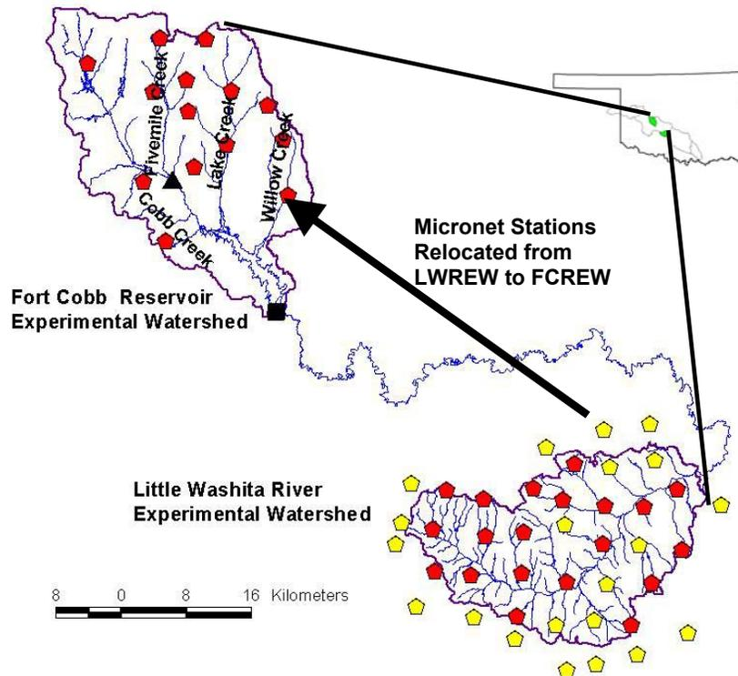
**Figure 3.** Research watersheds implemented in the prototype data system, showing configuration of the Micronet sites before and after relocation. (The triangle represents the USGS gage station near Eakly, OK, and the rectangle represents the OK Mesonet station at Fort Cobb Reservoir Experimental Watershed, used in Example 1 given below).
