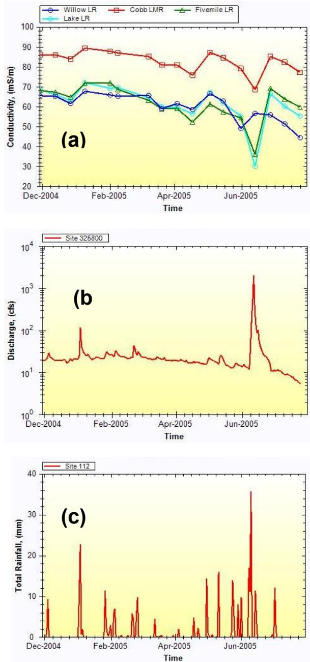
**Figure 5.** Time series of a) conductivity for four streams in the Fort Cobb Reservoir Experimental Watershed, b) stream discharge on Cobb Creek, and c) precipitation at Fort Cobb Reservoir Experimental Watershed.
