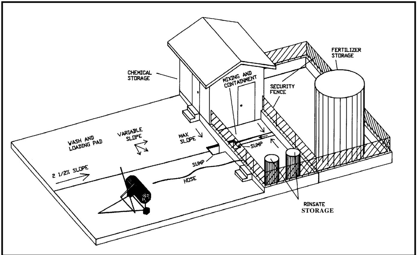
**Figure 1: Farm-sized fertilizer facility.** Source: *Modular Concrete Wash/Containment Pad for Agricultural Chemicals*, by R.T. Noyes and D.W. Kammel. *American Society of Agricultural Engineers Paper Number 891613.*
