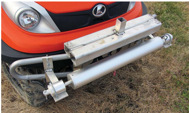
A vehicle-mounted passive gamma-ray sensor.
