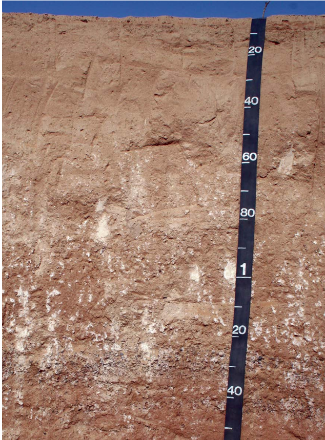
Masses of secondary calcium carbonate (white bodies below a depth of about 60 cm) in the calcic horizon of an Aridisol.
